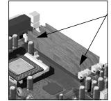
Each pair of memory sockets must contain identical memory modules (identical in size, speed, and type). That is, sockets **A1** and **B1** must contain identical modules, and sockets **A2** and **B2** must contain identical modules (or continuity modules).
